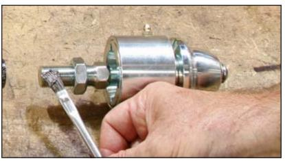
12. Screw pivot assembly into strut rod.
