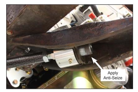
17. Tighten the backup nut using a 1/2"-drive ratchet; torque to 150 lb-ft.
