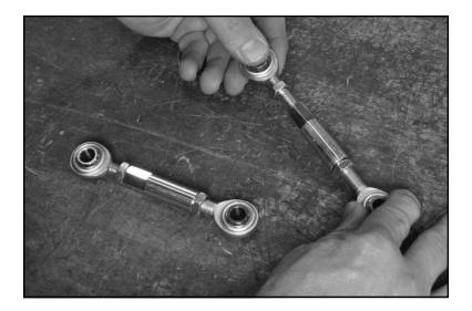
12. Attach the sliding-link clevis to each endlink assembly, using a 3/8" hex head bolt, two aircraft washers, and a locknut.
