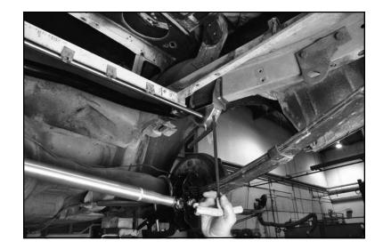
10. Assemble the endlinks. Thread the jam nuts onto the rod ends until there are 7-8 threads above the nut.
