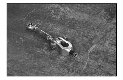
14. Attach the clevis onto the anti-roll-bar arms at the outermost detent. Tighten set screw, then jam nut. This position can be changed/ adjusted later, but we begin at this position as the baseline.
