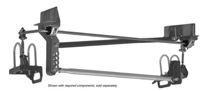
**Description:** Anti-roll bar with billet mounts for TCP Panhard Bar system. Features sliding endlink mount for anti-roll bar rate adjustment. Requires installation of TCP panhard bar system (TCP PHL-M10) and TCP driver-side leaf-spring plate (TCP PHS-M10).
