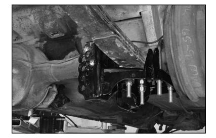
Install the TCP driver-side spring plate. Torque specification will depend upon U-bolt size. Continue with anti-roll bar assembly once all spring plate mounting hardware is tightened.
