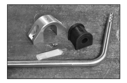
6. Slide the bushing over the bar and past the bend to the straight length between the two bends.
