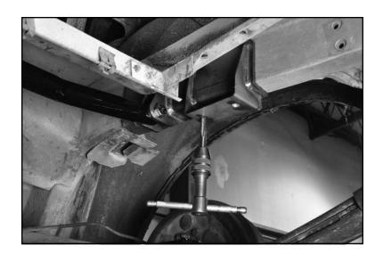
The bar can now raised into position and bolted to the frame brackets. Use two 3/8" socket head cap screws and two lock washers per mount.
