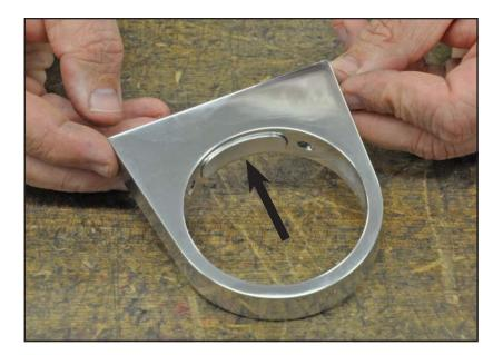
3. Slide the clamp assembly over the reservoir and tighten the allen head cap screws from the back side of the clamp. Test fit the reservoir to make sure the fittings are correctly clocked and easily accessible before fully tightening the clamp.
