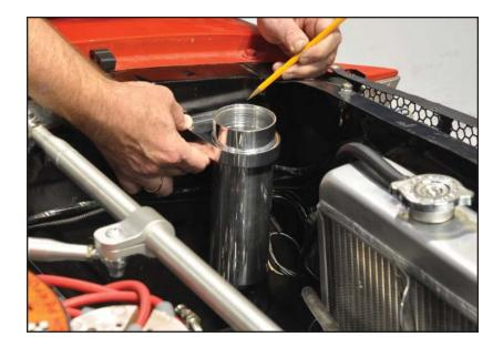
Use a ruler to measure the location of the two mounting holes in the adapter. The front hole is 15/16" back from the front edge of the adapter, and the rear hole is 2-15/16" back from the same front edge.
