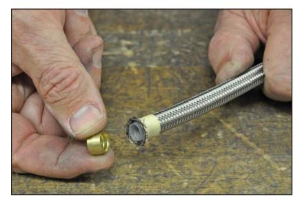
19. Place the brass ferrule in between the Teflon hose and steel braid as shown.
