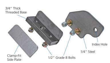
clamp is used to sandwich the factory frame rail between the base assembly and loose plate. This ensures a perfect bracket fit and eliminates the possibility of filling gaps around the bracket when welding. The clip assembly is secured to the welded chassis brackets by eight 1/2" Grade 8 bolts.
