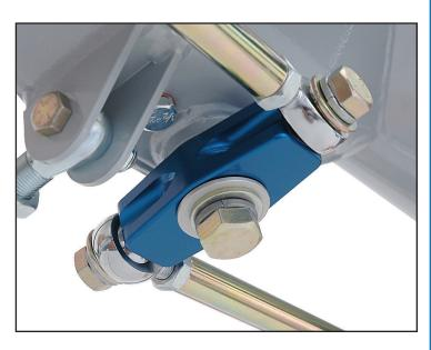
used for its excellent strength and light weight. The pivot rotates on a press fit, sealed roller bearing, secured by a retaining ring. A 3/4" Grade 8 bolt secures the pivot assembly to a specially designed broad based mounting bung welded directly to the bottom of the FAB9™ center section.
