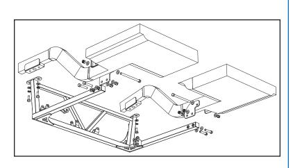
installer error. The rear clip assembly and subframe connector support are then bolted securely to the mounting brackets and weld-in subframe connectors. The remaining suspension components simply bolt to existing mounts on the rear clip assembly, subframe connector support, and rear end housing. To guide you through each step of installation, setup, and fine tuning, a detailed, illustrated instruction manual is provided with each kit.
