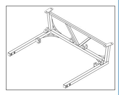
by 3/16" thick sheet metal gussets. Each piece of tubing is capped to improve torsional strength and to prevent moisture from entering the assembly. Vertical uprights are fitted with stout 1/4" thick mounting plates with slotted holes to allow for chassis variances during installation. Clip frame rails are capped at their leading edge and fitted with two bolt sleeves to prevent the tube from collapsing when mounting hardware is tightened.
