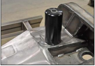
The surface mounting method provides the cleanest of install options with the canister displayed or hidden away and the hoses and vent hidden from view.
