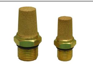
A large -8 sized sintered bronze breater vent is used instead of the more commonly found -6 size. The increased surface area and port volume improves vent flow without increasing air velocity.
