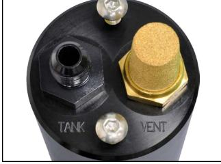
The canister base features the two mounting screws as well as o-ringed ports for -6 hose attachment and the -8 sintered vent. Each port is clearly labeled.
