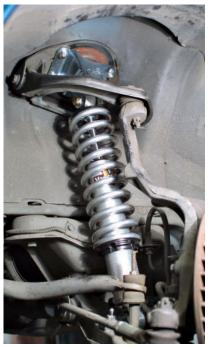
We have to admit that we sort of dig this bolt-on coilover conversion for fourth-gen Camaros. The bracket at the top attaches to the A-arm mount like a stock setup. According to Alston, the "extra-long" shock allows for extensive choices of ride height, spring rate, and shock valving.
