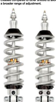
The company's coilover shocks and struts feature the same quality of construction as their factory-replacement bolt-in Varishocks but allow spring preload adjustment and spring rates to be more easily changed. Preload, in case you were wondering, is required to position the shock at the correct ride height length.
