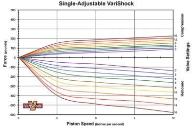
Single-adjustable shocks are pretty straightforward. By turning the knob, you either increase or decrease both rebound and compression damping. This is illustrated by this graph from Alston's shock dyno. As you can see, however, the rebound damping increases more than the compression damping—there's a usable range of adjustment, making a single-adjustable shock far superior to a nonadjustable one. It is limited, however, since both shock actions are adjusted together through 16 settings.
