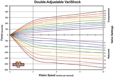
This is illustrated to good effect on this second graph from Alston's shock dyno. As you can see, there's a much greater range of adjustment to be had. Better yet, since the two are independent, it's possible, for example, to adjust rebound damping (coming apart) to full soft and compression damping (coming together) to full firm. That's an extreme example, but the bottom line is that you've got access to 256 possible combinations—meaning the right one is in there somewhere.
