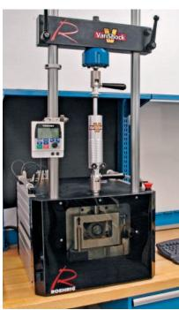
Chassisworks makes extensive use of its state-of-the-art shock dyno for research and development. Every VariShock is also tested and calibrated to strict performance guidelines before it's shipped to the customer, ensuring that each shock performs as it should.
