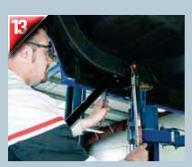
Control arm (trailing arm) fasteners are torqued to 60 lb-ft. Make sure the grease jerks are accessible before tightening.
