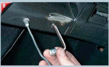
This is how to install the 1/2-20x5x3-inch U-bolt, which attaches the subframe to the frame rail. Richard uses a magnet to guide the U-bolt. Once in place, we're ready for subframe installation. Be careful never to lose this U-bolt inside the frame rail. Position the subframe and install flat washers and locknuts. Locknuts are torqued to 30 lb-ft.
