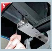
When you have committed to a location and are positive about measurements, scribe the holes and edges as shown. Be absolutely certain about location before drilling and welding.
