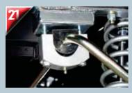
The adjustable 5812-M10 g-Bar sliding-link anti-roll bar dramatically reduces body roll. Secure the mounts as shown using \$^1\_6-16x2^1/2-inch bolts and lock washers. Torque for these fasteners is 30 lb-ft. Use poly-lube on the urethane bushings during installation.
