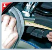
With the subframe positioned and C-clamped in place, get your measurements. There should be exactly 10 inches from the trailing edge of the subframe bracket to the leading edge of the rebound bumper bracket. If measuring from the leading edge of the rebound bumper bracket to the leading edge of the rebound bumper bracket to the leading edge of the subframe bracket, it should be 4-1/4 inches.
