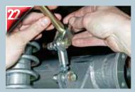
Assemble the bar ends as shown, slipping each end into the adjustable link. Leave five to seven threads showing between the jam nut and link end.
