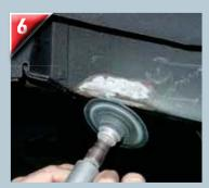
Remove the paint and undercoat where uou intend to weld. The Restomod Shop suggests welding in addition to bolting for a secure installation.
