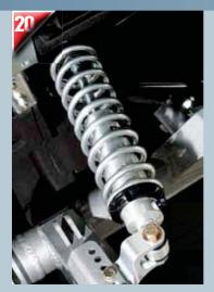
VariShocks should look like this once they're installed. Bolt hole positioning at the lower mount determines ride height.
