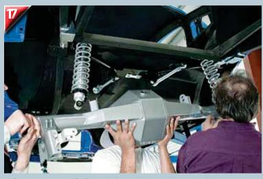
Chris Alston's FAB-9 housing is attached at the shocks and lower control arms. The FAB-9 makes our TCP package complete and ready for anything.
