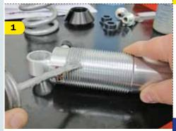
The TCP coilover shocks come unassembled and will require some basic prep before they can be installed. First, a liberal coat of antiseize is applied to the shock's threads in preparation for installing the adjustable spring seat.
