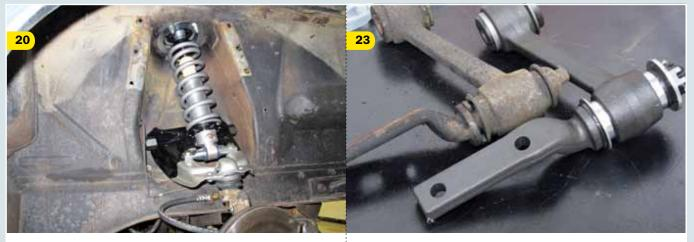
With the coilover installed you can see how simple, yet effective, the TCP coilover kit is. The double adjustable configuration of our shock setup means we have two separate adjustment knobs. We decided to face them inboard for access through the center of the upper control arm. You can easily rotate the shock body to face the knobs towards the tire if you wish.
