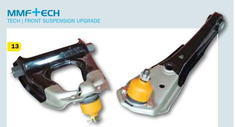
A quick call to Mustangs Unlimited solved our ball joint problem. Mustangs Unlimited suggested Scott Drake's new show-quality control arms. While far from a show car, these new control arms are built with OE level steel in the right thickness with high-quality riveted ball joints—just what the High School Hauler needs!
