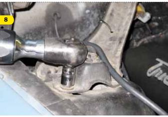
With our shocks assembled, we can now move forward with disassembly of our stock components-mainly the shock and coil spring. Remove the shock mounting cap retaining nuts (the mounting caps will not be reused). We're installing TCP's Tower Export Brace kit as well, so we're removing the stock braces at this time, too.
