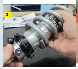
Thread the spring seat onto the shock from the top and follow the spring seat with the coilover spring, seating it onto the seat.
