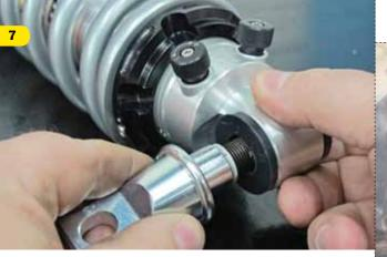
Add the aluminum crush washer to the cross-shaft half with the set screw in it and press it into the shock end. Press the other half of the cross-shaft into the opposite shock end, and while applying pressure to the cross-shaft, thread the two halves together until they seat and then tighten the two halves until they're even.
