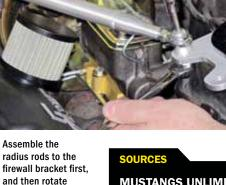
firewall bracket first, and then rotate the rod (hold the loose rod-end to maintain even thread engagement) until the rod-end lines up with the shock tower mounting hole and
