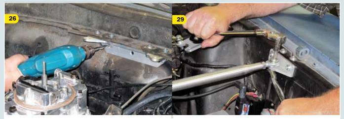
You will have to drill the three holes for the horizontal bolts, ensuring the firewall is clear of any wiring before you do so. It'll take a second set of hands to slip the support plate up under the dash and hold the retaining nuts while you tighten the bolts from the engine bay side.
