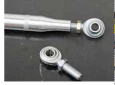
equal amount of threads/turns. The zinc-colored nut is for the left-hand threaded rod-end, which is threaded into the radius rod end with the knurling on it, shown here.
