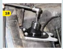
TCP offers these polished coilover mount covers if you're looking to add a little shine to your installation. They install easily by removing the coilover's grease fitting and securing the mount cover with the included Allen screw into the grease fitting hole.
