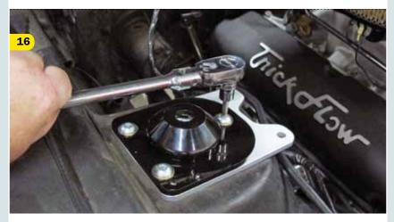
The coilover upper mount sandwiches the shock tower. The upper plate is placed over the shock opening while the backing ring is installed from inside the shock tower. If you're installing TCP's Tower Export Brace kit as well, you'll have to decide whether you want the mounting plate above or below the coilover plate. Mounting it below, as we have, lowers the front suspension approximately another ½-inch.
