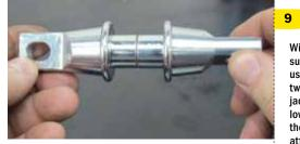
screw seats and measure the gap, if any. You want less than 0.070-inch gap. As confirmed here, our cross-shaft assembly was in spec.
