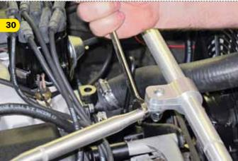
The truss support brace kit is a nice option, tying the Monte Carlo bar kit into the Tower Export Brace kit with a second pair of radius rods that attach to the shock tower plates.
