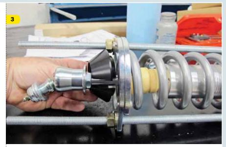
With high-rate front springs, it's often a little difficult to install the upper spring seat. The easy solution is a spring compressor. TCP offers a nice, simple compressor that works easily by registering on the lip of the lower spring seat and compressing the spring as shown. Compress the spring just enough to slip the upper spring seat into place and back the compressor off to seat the spring fully.
