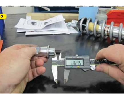
The TCP cross-shaft uses a large set screw to assemble the two halves. Following the directions, the two halves are chased with a  $\frac{1}{2}$ -20 tap and then the set screw is threaded into one side. Measure the remaining set screw protruding to verify it is between 0.525 and 0.625-inch. We had to grind ours down slightly to get it within spec.
