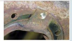
separate the mount from the shock tower. Grind any remaining spot-weld burrs flush and add a shot of paint to the bare metal.
